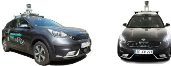
Fig. 2. One of the KIA Niros, which has been automated at FH Aachen.
