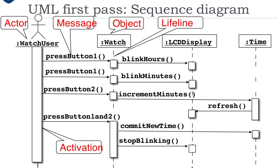
Sequence diagrams represent the behavior of a system as messages ("interactions") between *different objects*
