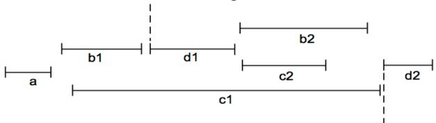
Discriminator makes sure that d2 only enabled after c1 of first iteration completes
