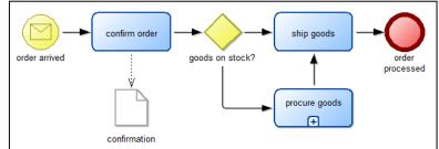
A model contains instances of the concepts defined in the meta-model. The object "confirm order" represents a real entity; it is an instance of the concept «task"
