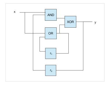
1. Model the behaviour of the circuit as a transition system assuming that the initial state of the registers is 0.
