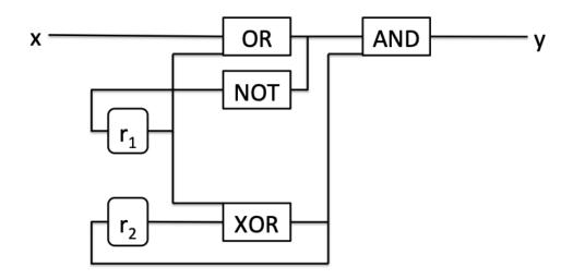
Draw the transition system describing the behaviour of the circuit. Use  $AP = \{y\}$  as set of atomic propositions to label states. Registers are initialised to 0.
