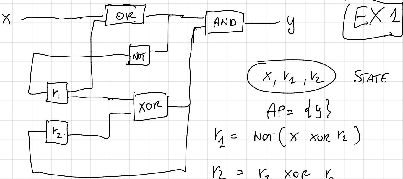
$$y = (r_2 \text{ XOR } r_2) \text{ AND } (x \text{ OR } r_1)$$
