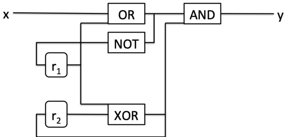
Draw the transition system describing the behaviour of the circuit. Use  $AP = \{y\}$  as set of atomic propositions to label states. Registers are initialised to 0.
