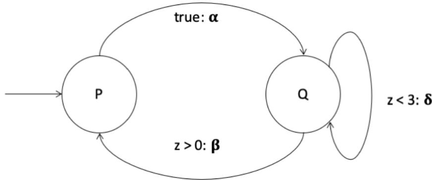
where  $z$  is a variable such that  $\text{dom}(z) = \{0, 1, 2, 3\}$ ,  $g_0 \equiv (z = 1)$ ,  $\text{Loc}_0 = \{P\}$ ,  $\text{Effect}(\alpha, \eta) = \eta[z := 0]$ ,  $\text{Effect}(\beta, \eta) = \eta[z := \eta(z) - 1]$  and  $\text{Effect}(\delta, \eta) = \eta[z := \eta(z) + 1]$ .
